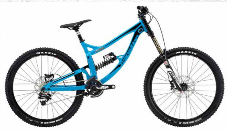
TR500 TRAVEL: 180MM OR 203MM / WHEEL SIZE: 27.5" OR 26"
