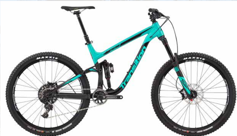
PATROL TRAVEL: 155MM REAR 160MM FRONT / WHEEL SIZE: 27.5"
